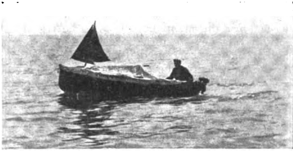
At Times It Was Difficult to See the Sea Pup. So the Sail Shown Above Was Rigged and Was Always Visible Even When the Boat Was in the Trough of the Waves
